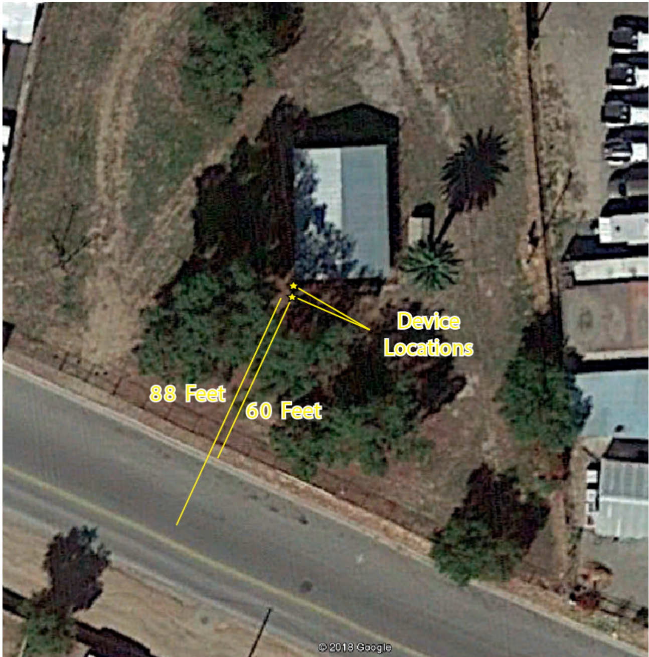
Figure 2: Site view of Trujillo Adobe showing Geovision seismographs at the southwest corner and the 60' distance to edge of Center Street and 88' distance to center of nearest travel lane. (from Google Earth Pro)
