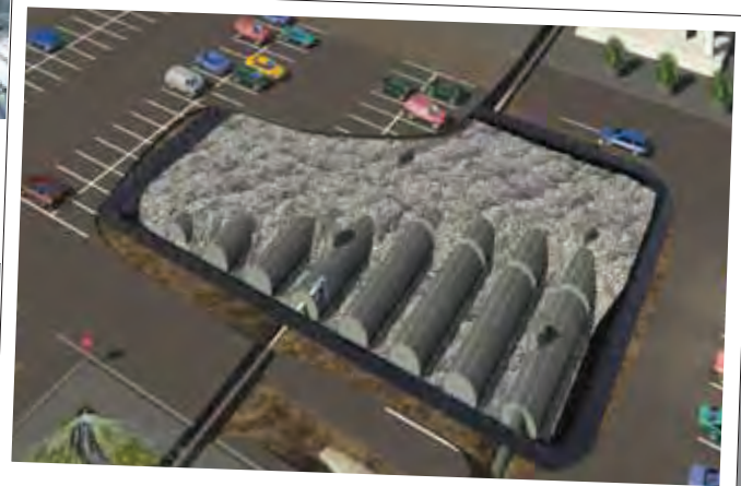
Stormwater runoff is stored in the pipe and surrounding stone
