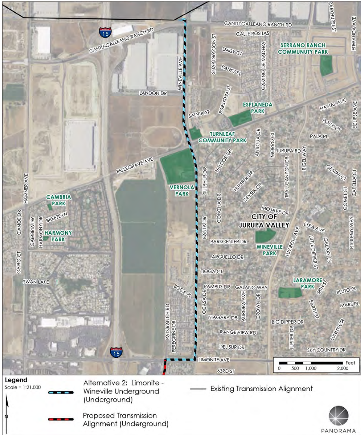
Figure 4.2-2 Alternative 2: Wineville – Limonite Underground
