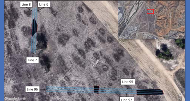
Figure 7: GPR Lines 6-8 and 95-97 taken on August 28th, 2018 and July 18th, 2018 respectively at Pellissier Ranch. Black shapes outlined in red denote locations of anomalies seen in profiles. The anomaly between Lines 6-8 represent a potential collapsed structure. Anomalies between Lines 95-97 represent (from west to east) a 7 meter wide canal and a 30 meter long, abruptly interrupted reflector.
