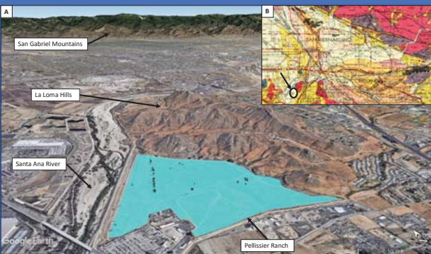
Figure 1: A) The Pellissier Ranch site (aqua) in Colton, CA. Viewed at an angle to the northeast to emphasize the absence of topography across the site and the San Gabriel Mountains. B) Geologic map of San Bernardino County, CA. Pellissier Ranch is circled. Quaternary wash deposits dominate the entire site. La Loma Hills are composed of Cretaceous quartz diorite. The San Gabriel Mountains, where the Santa Ana River originates, are composed of Cretaceous or Jurassic quartz monzonite.
