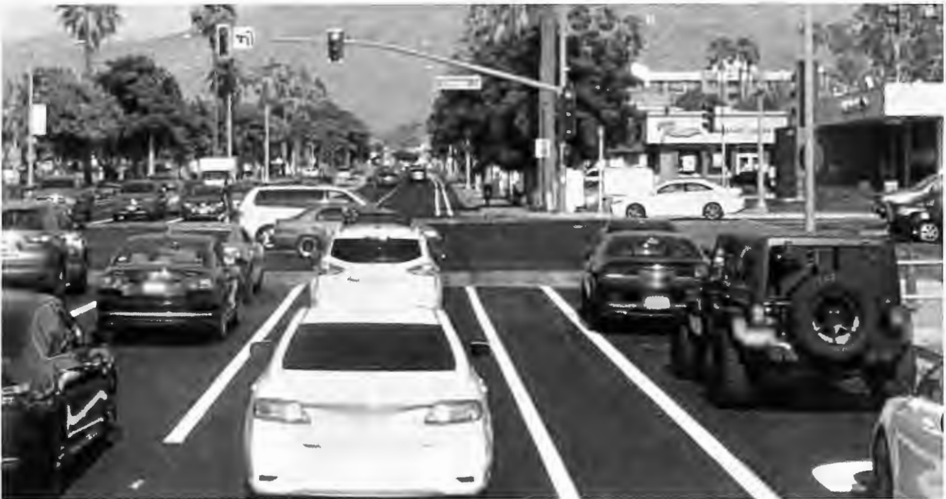
Intersection 4 – Chicago Ave & University St - Looking eastbound. Improvements include –green bike lane striping & audible pedestrian pushbuttons.
