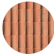
NEW ROOFING MATERIAL SHALL BE SPANISH-STYLE CLAY TILE, RATED FOR MIN. 100 MPH WIND LOAD. SHALL BE APPLIED PER MANUFACTURER SPECIFICATIONS OVER ONE LAYER OF #30 FIRE-RATED FELT. SHEATHING TO BE 15/32" OSB OR CDX PLYWOOD TO MATCH EXISTING. TILE COLOR TO BE AGED CHESTNUT OR EQUIVALENT, CLASS A FIRE-RATED.
