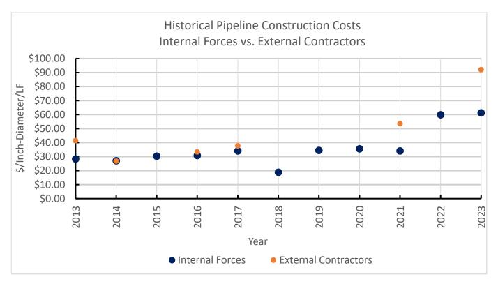
Based on the data analyzed, utilizing internal forces for water pipeline construction projects proved to be very cost effective compared to hiring external contractors. On average, over the period reviewed and for the years where comparative data is available, projects completed by external contractors were approximately 29% more expensive than those completed by internal crews.
