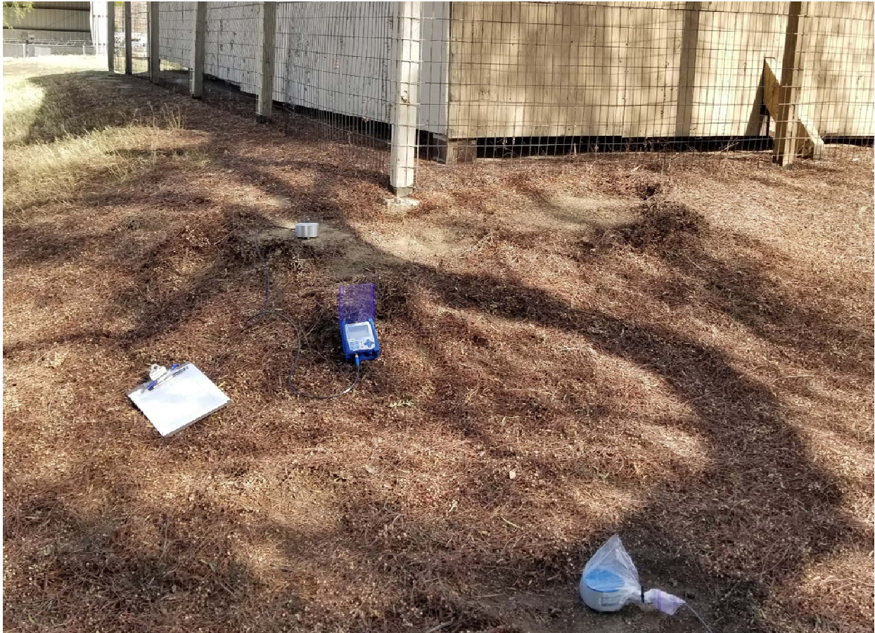
Figure 1: Photograph of the seismograph installations near the SW corner of Trujillo Adobe
