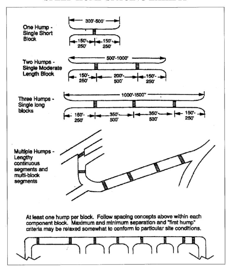
Figure 4.10. Spacing of speed humps.
