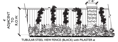
C TUBULAR STEEL VIEW FENCE (BLACK) with PILASTER at DETENTION BASIN 5'-6" HIGH
