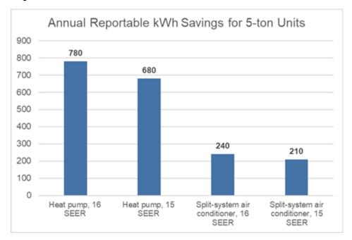
The table below outlines lifetime kWh savings of a 5-ton heat pump unit by SEER rating:
