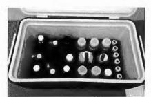
Sample containers for all analyses except certain microbiological methods are purchased in batches, precleaned by each vendor according to EPA guidelines. Every batch is associated with a lot number, identified on each container and tracked to trace any contamination that might originate with the vendor. All Volatiles and Metals lots are tested additionally at Eurofins to verify the absence of
