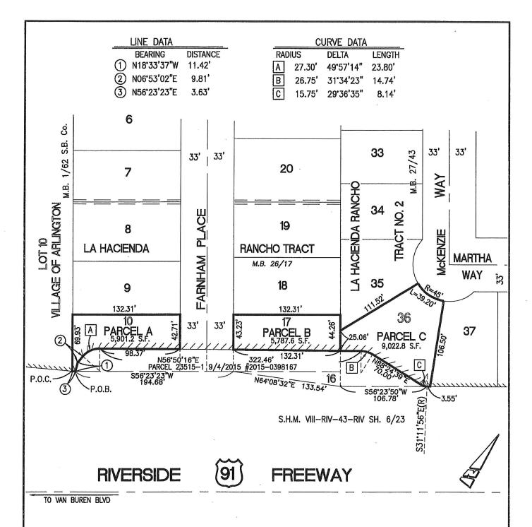
BEARINGS AND DISTANCES SHOWN ARE BASED ON CALIFORNIA COORDINATE SYSTEM OF 1983, ZONE 6 MULTIPLY DISTANCES SHOWN BY 1.000033361 TO OBTAIN GROUND LEVEL DISTANCES.
