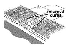
Curb ramps with returned curbs do not have flared sides and a parking citation is only issued when the actual ramp is blocked. Vehicles may park on the street up to the portion of the curb where the vertical curb begins.
