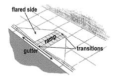
The area cut down for the curb ramp begins at the portion of the curb where the slope of the flared sides descends towards the middle of the ramp where it meets the gutter. A vehicle parked blocking any portion of this area is in violation of CVC 22500(I) as it reads: In front of or upon that portion of a curb that has been cut down, lowered, or constructed to provide wheelchair accessibility to the sidewalk. Vehicles parked in this area may be cited.
