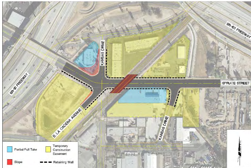
Spruce Street Grade Separation – Alternative 2
