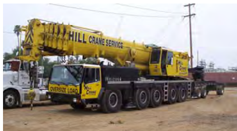
CRANE USED TO SET STEEL POLES
