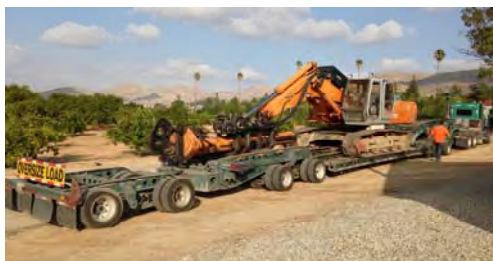
DRILL RIG ON TEN AXLE TRAILER
