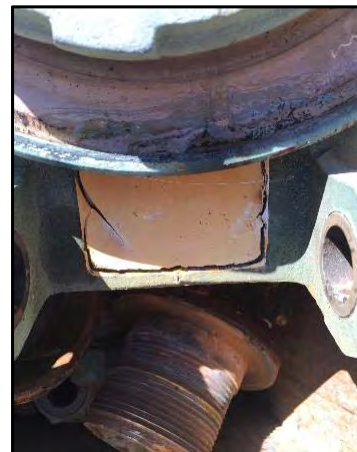
Typical Cracked Epoxy Seal in the Counterweight
