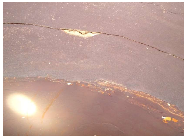
Circumferential pipe crack
