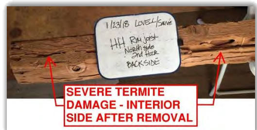
Figure 14 – Back side of Second Floor rim joist after being removed (January 23, 2018)
