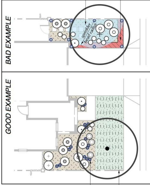
*Overhead irrigation, such as sprinkler heads, installed in a sparsely planted landscape results in inefficient water management by applying water to non-planted areas.*
