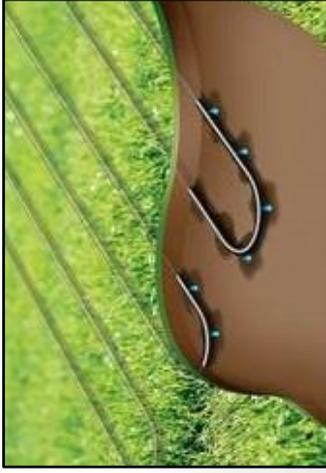
*Subsurface drip line irrigation can be used for a wide variety of planting situations. It is one option for narrow parkways or a planted 24" setback area from non-permeable surfaces.*
