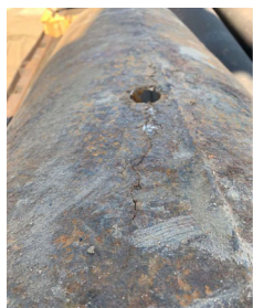
Holes and cracks on the existing Scheuer Well Supply Main
