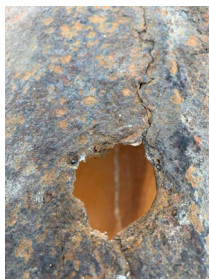
Holes and cracks on the existing Scheuer Well Supply Main
