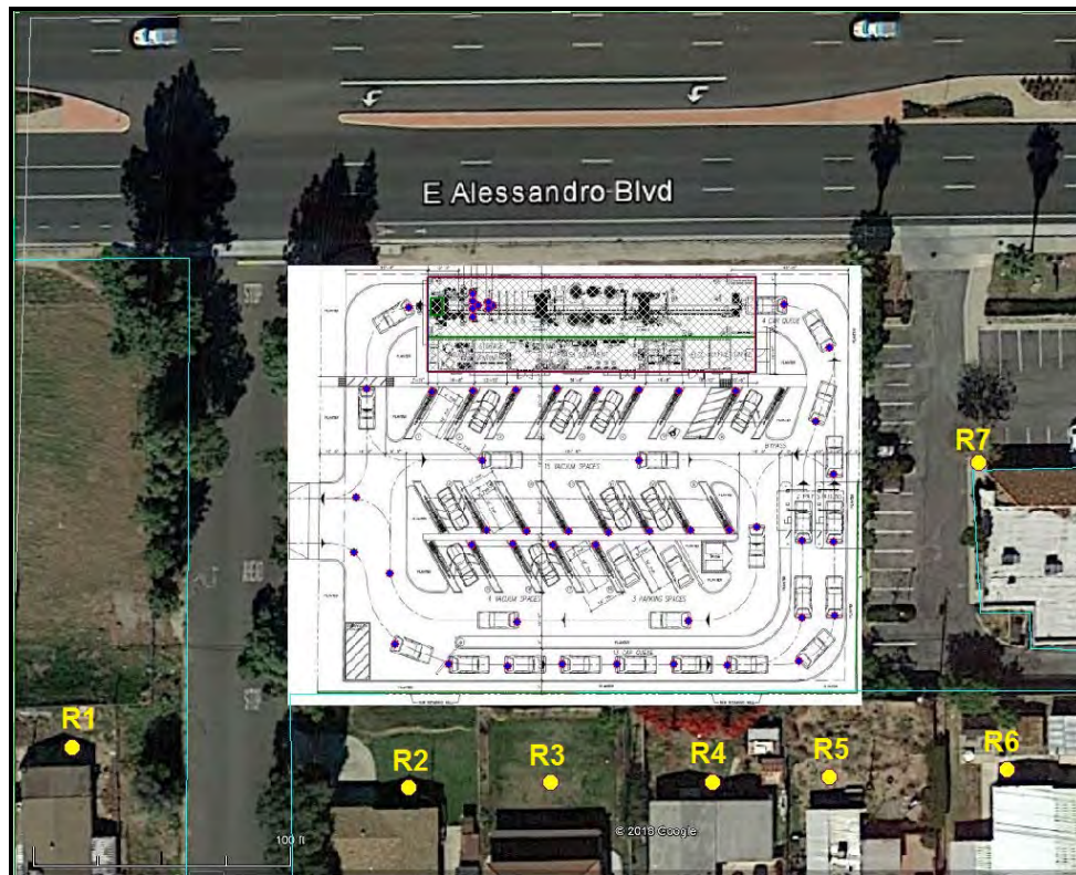
Figure 6. Proposed Express Car Wash Layout with Receptor Locations
