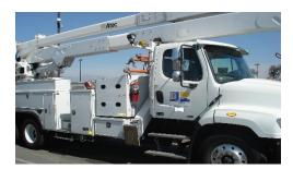
Two (2) of the new Digger Derricks are equipped with an auger (drill) that can create large holes for setting poles; they are specifically designed for heavy work and are capable of pulling and hauling thousands of
