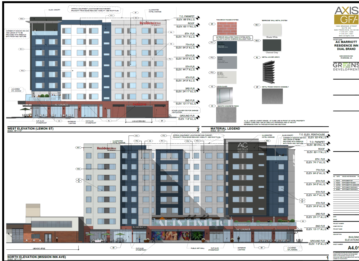
Figure 2: West and North Elevations
