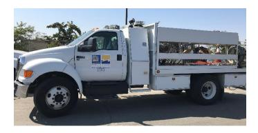
The new Ford F550 will replace the same from 2013; however, the replacement model will include a hybrid engine, ensuring that RPU remains compliant with Southern California Air Quality Management District (SCAQMD) guidelines. This is ideal when out-of-hours work is required in residential areas, particularly at night, as its quiet engine will not cause disturbance to residents. The picture below shows vehicle Asset Number E429, the current F550.
