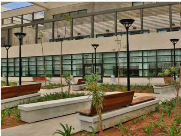
Examples of passive barriers including kneewalls, planters, and public seating integrated into low retaining walls
