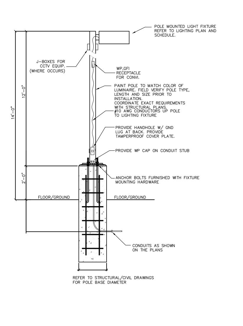
14' POLE & BASE DETAIL (TYPE SC1S & SD1S) | SCALE | NTS
