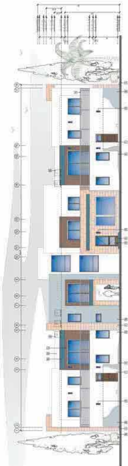
FRONT (EAST) ELEVATION 3/16" = 1'-0"
