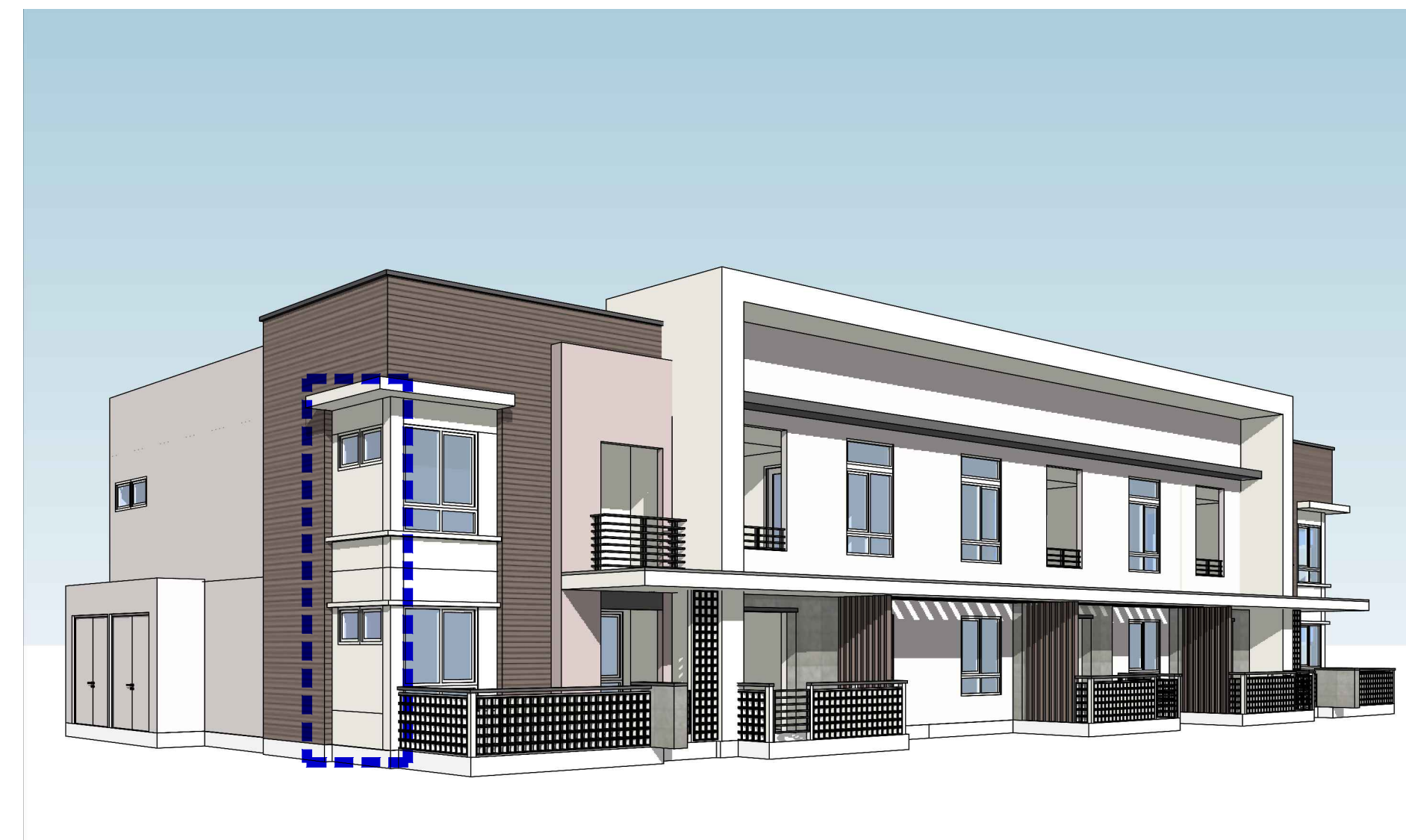
VIEW OF TYPE A SIDE ELEVATION W/ TRANSOM WINDOW SPECIAL CONDITION WHEN FACING SINGLE FAMILY RESIDENTIAL HOMES
