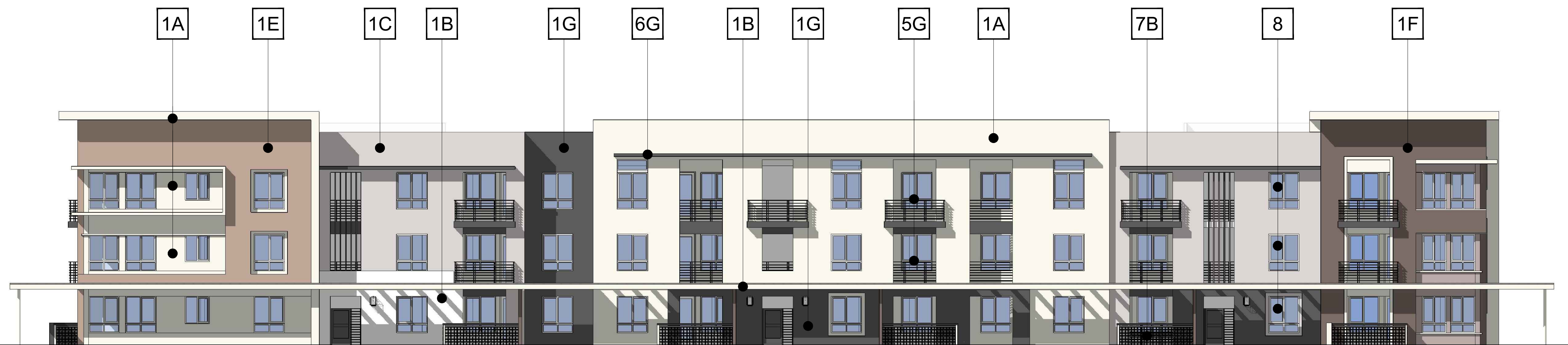
TYPE III - ALL-STUCCO ELEVATION
