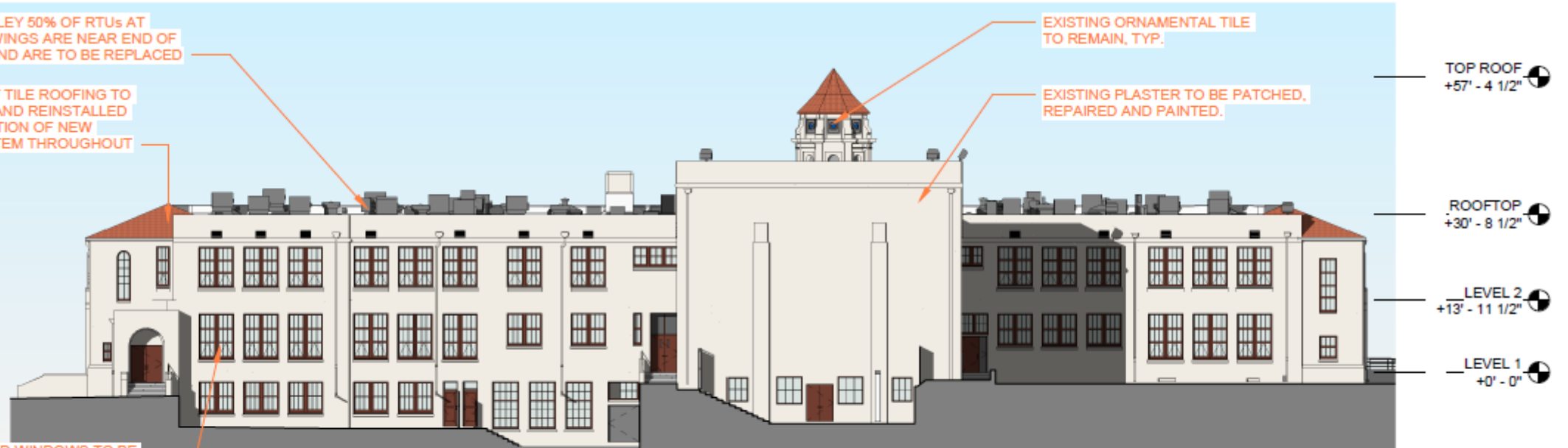
2 PROPOSED SOUTH ELEVATION 3/64" = 1'-0"
