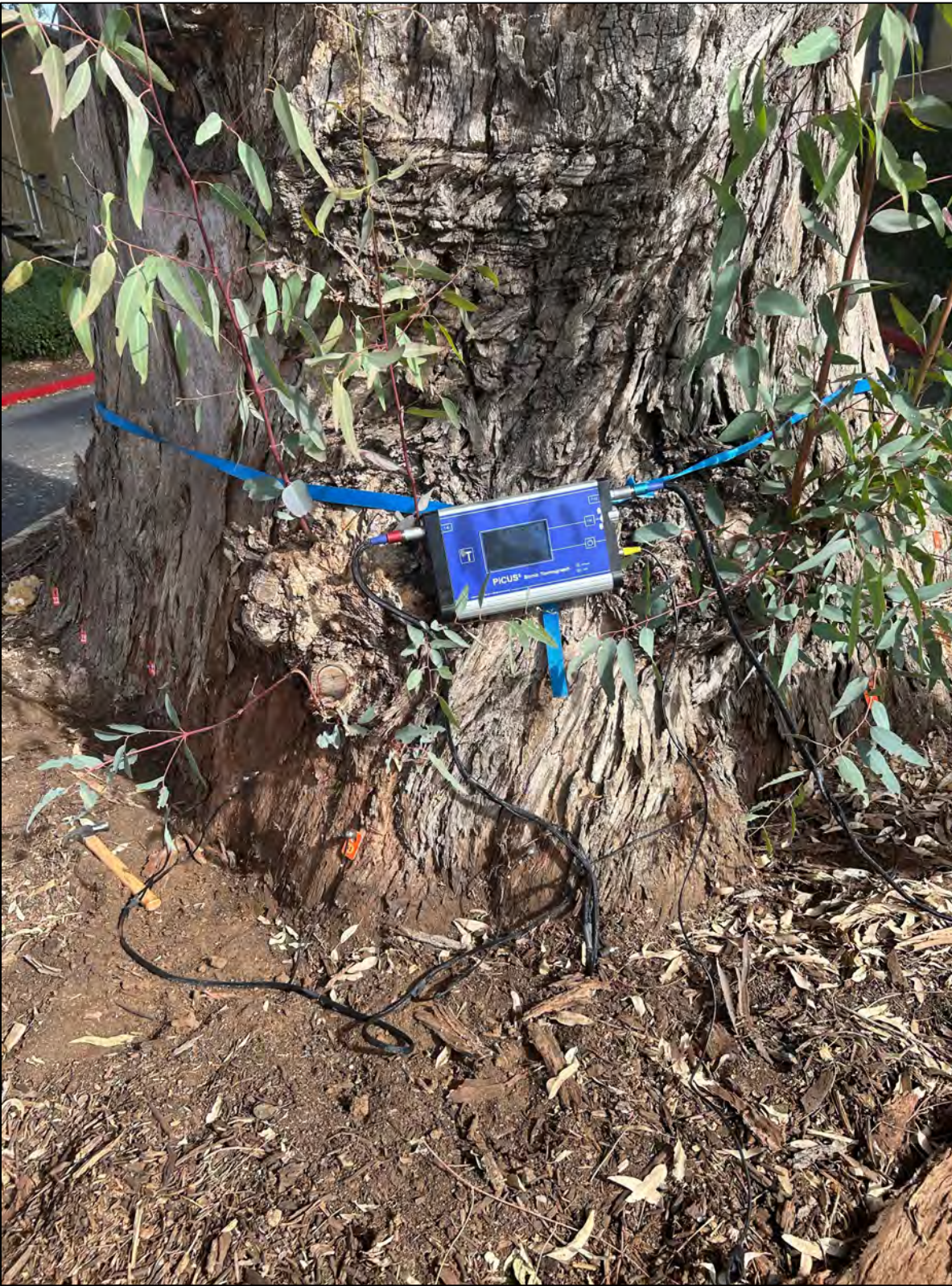
Figure 10: Drilling points 23 - 30 and the PiCus 3.
