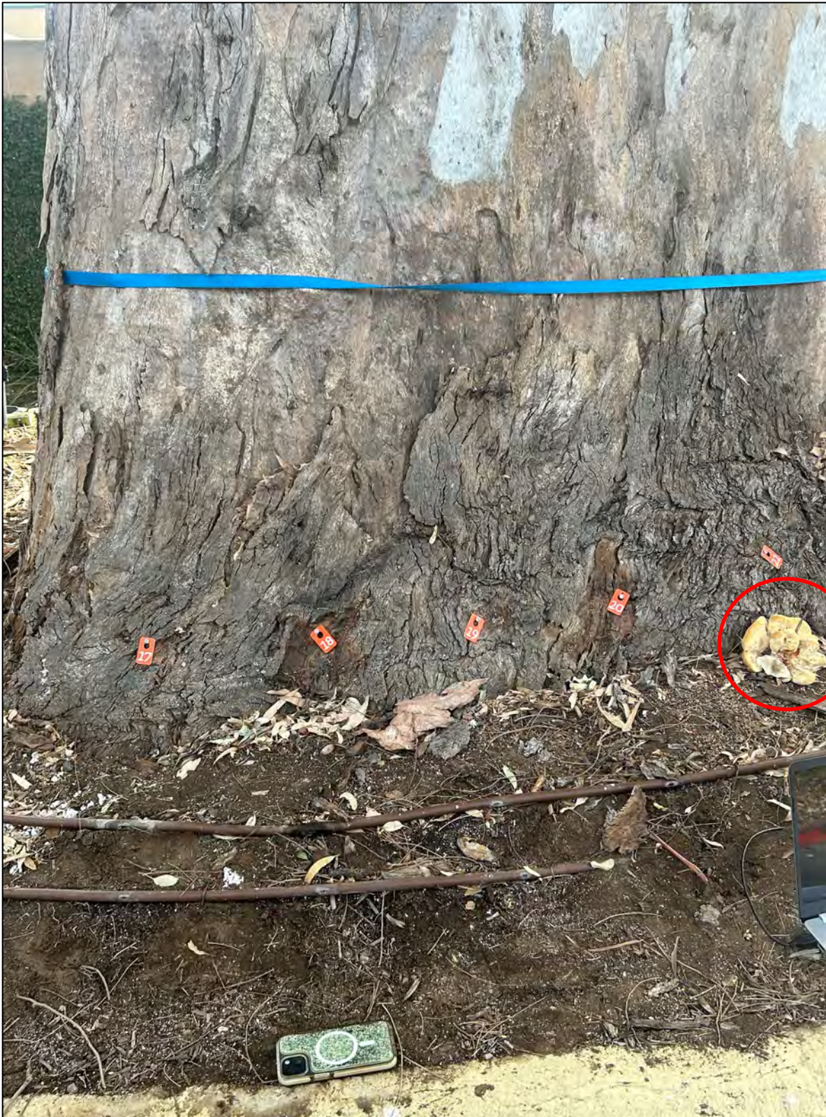
Figure 7: Drilling points 17 - 21 and a fungal conk.
