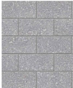
BURNISHED CMU LIGHT GRAY OCCURS AT RESIDENTIAL PATIOS - GROUND LEVEL
