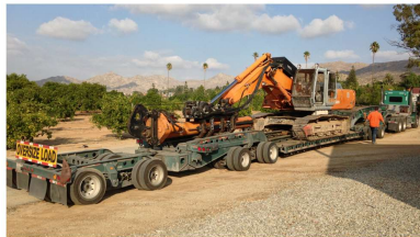
DRILL RIG ON TEN AXLE TRAILER
