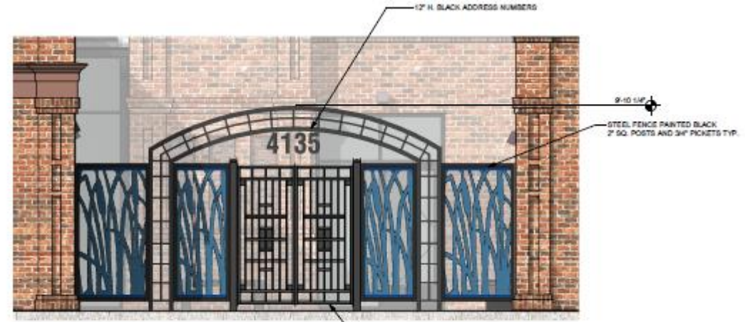
1 ENTRY GATE AT MARKET ST. SCALE: 3/8" = 1'-0" STEEL ORNAMENTAL ENTRY GATES AND ARCADE FEATURE PAINTED BLACK TYP.
