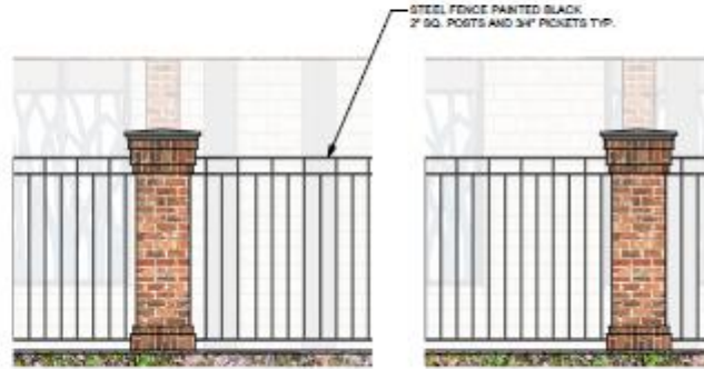
2 STEEL FENCE ELEVATIONS SCALE: 3/8" = 1'-0" OCCURS AT WEST AND NORTHWEST PROPERTY LINES AROUND PARKING AREA
