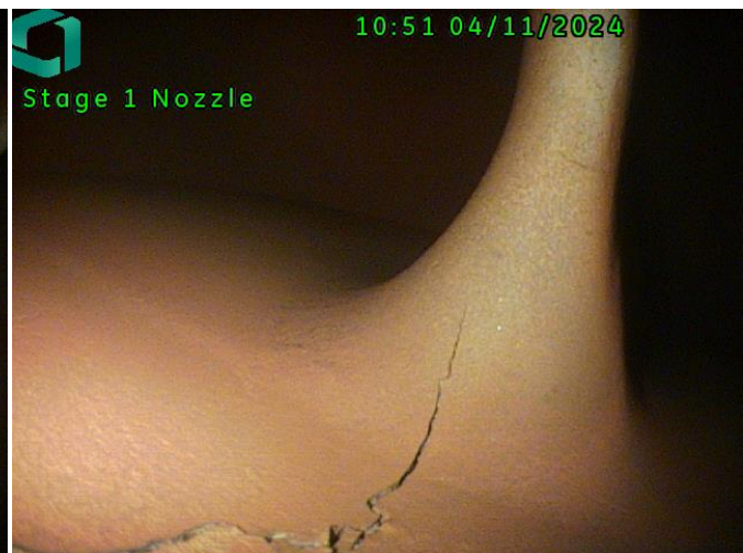
Figure 3. Stage one nozzle - flume crack
