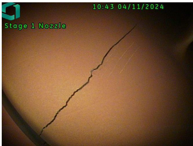
Figure 2. Stage one nozzle - lateral crack
