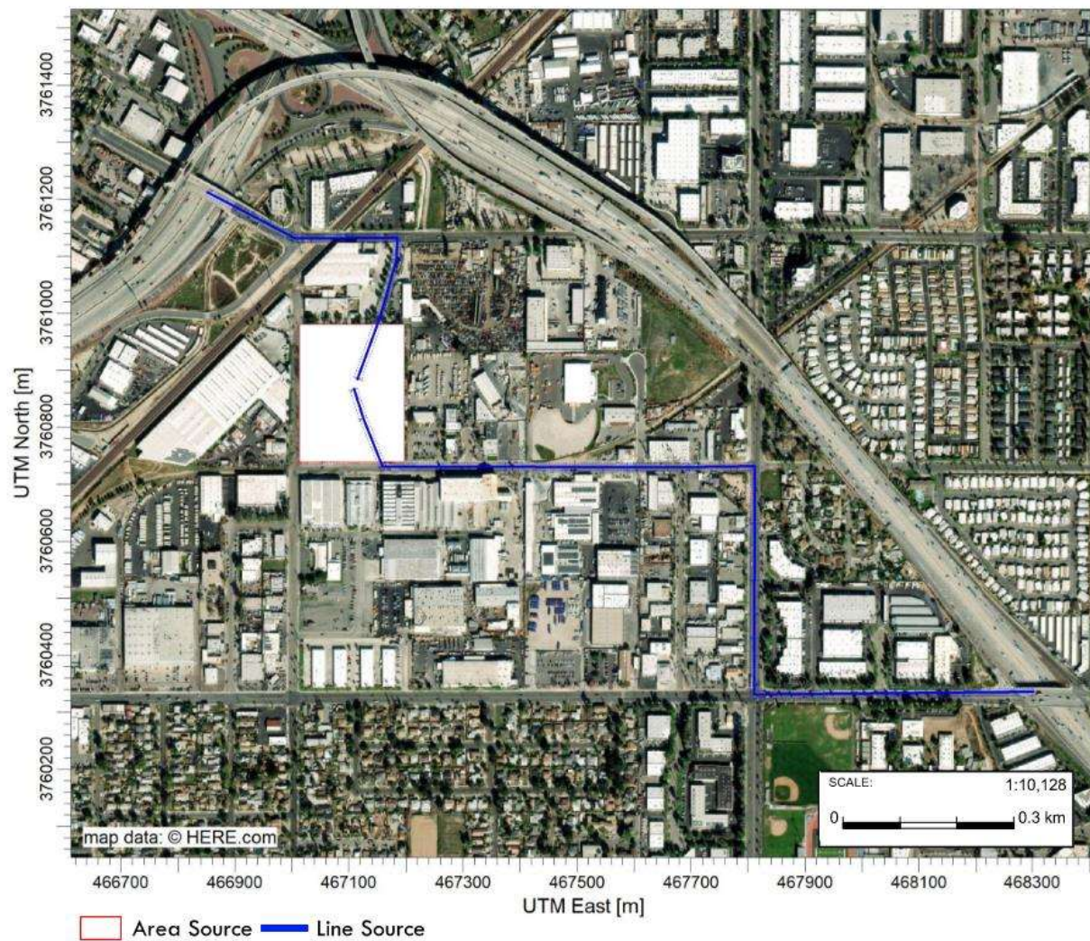
Figure 3: Locations of the Project's Construction On-Site and Off-Site DPM Emission Sources
