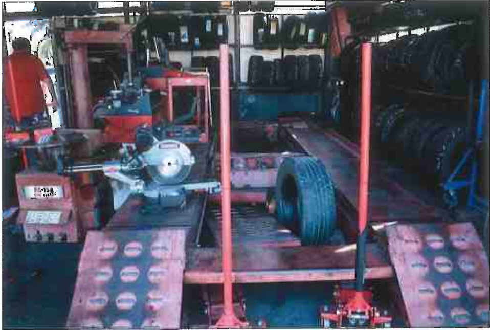
#9 The above ground lift.
