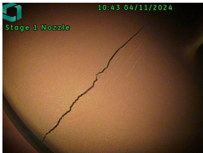
Figure 2. Stage one nozzle - lateral crack
