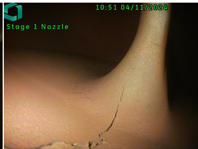
Figure 3. Stage one nozzle - flume crack
