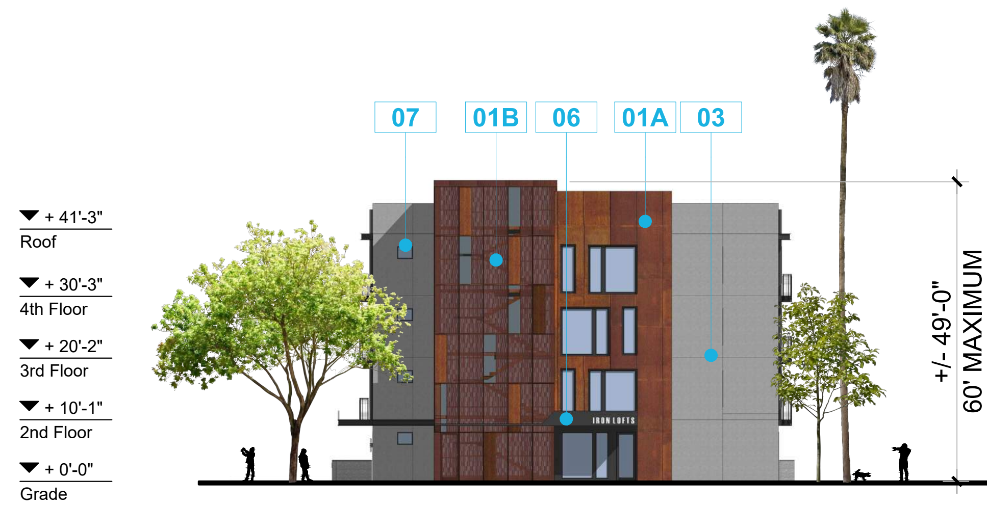
4B. BUILDING A - PARTIAL EAST ELEVATION (LEFT)
