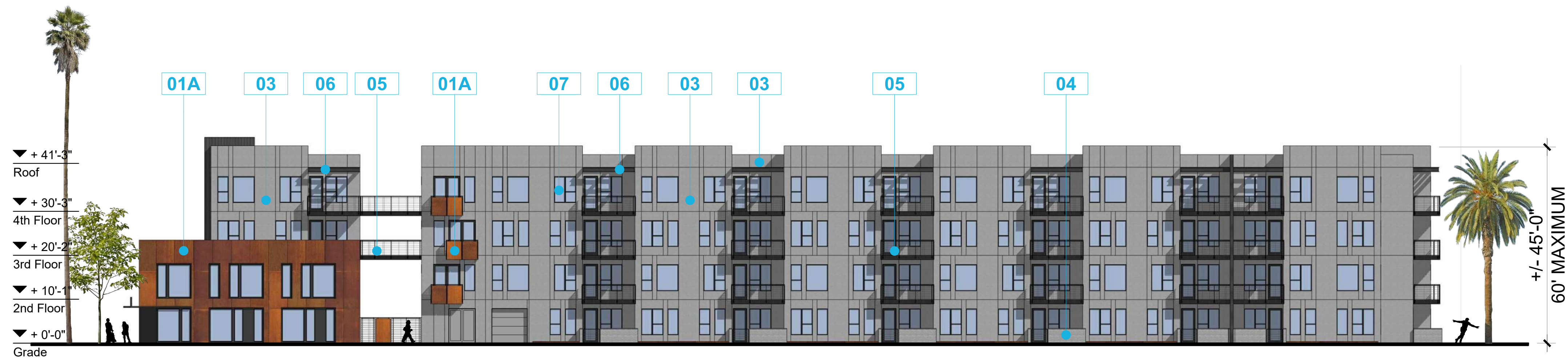
4A. BUILDING A - PARTIAL EAST ELEVATION (CENTER)
