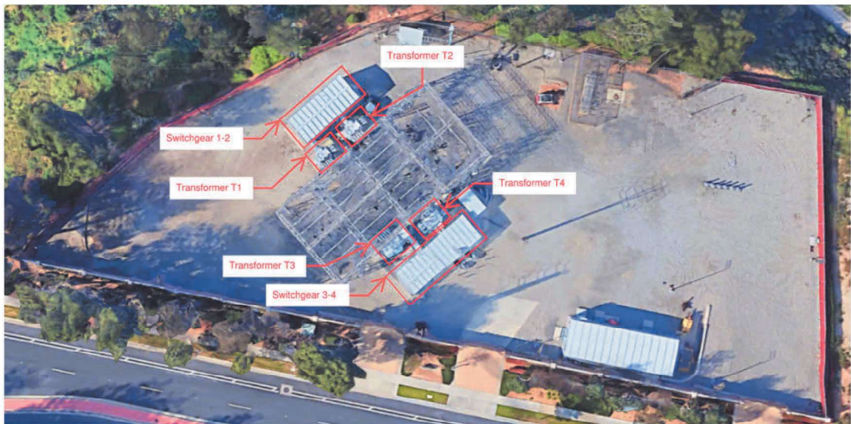
Figure 1: La Colina Substation Plan View
