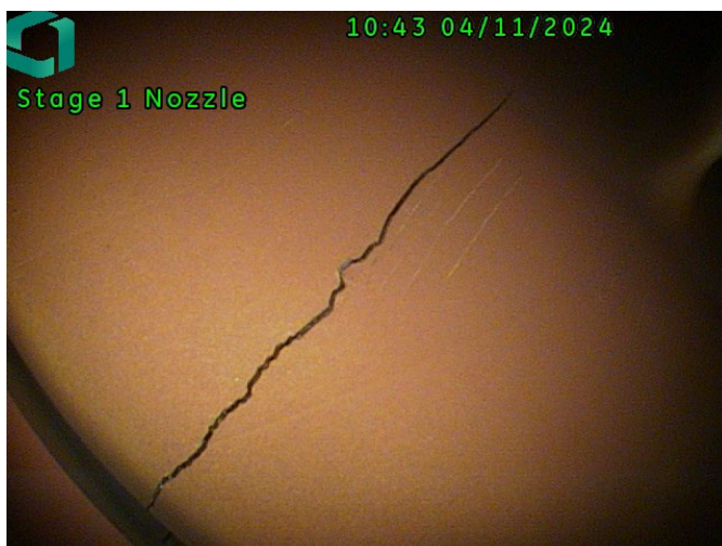
Figure 2. Stage one nozzle - lateral crack
