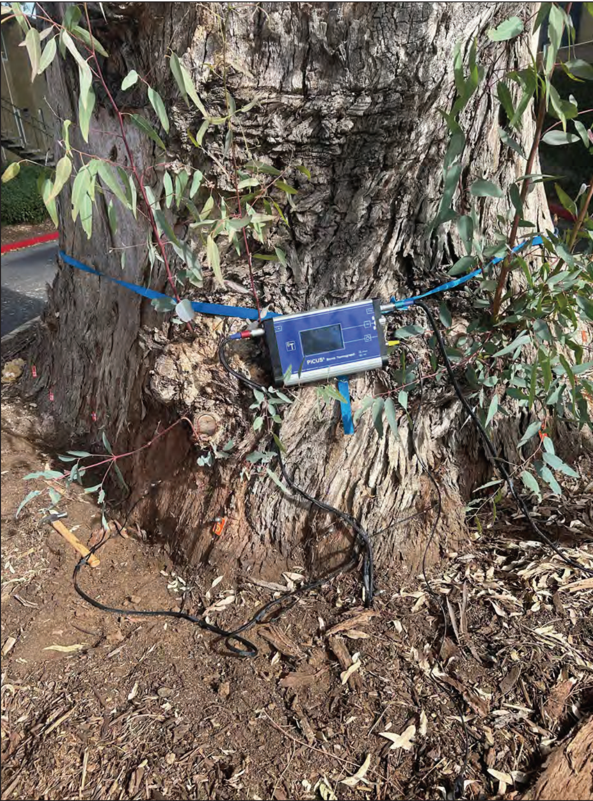
Figure 10: Drilling points 23 - 30 and the PiCus 3.
