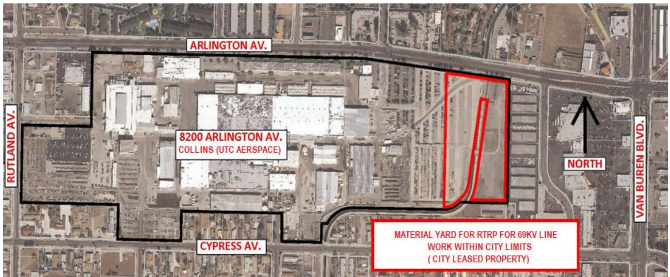
Material Yard to support RTRP 69kV sub-transmission lines work
